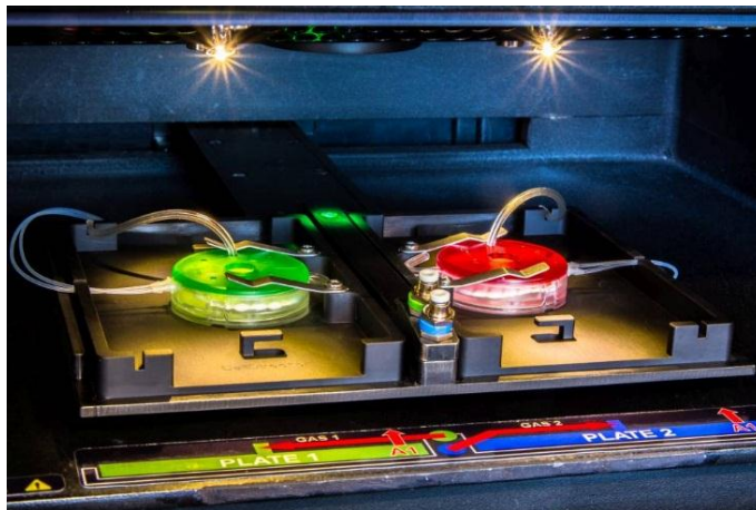
Figure 1. Cell-IQ® incubator loaded on the left plate holder with a CellDirector®2D (green) and the right plate holder with a CellDirector®3D (red).
