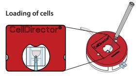
The cell-matrix mixture is injected into the cell culture chamber with a standard pipette through the cross-shaped slit.
