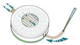
Cells are seeded in a single step by injecting the cell suspension through the outlet tube.
