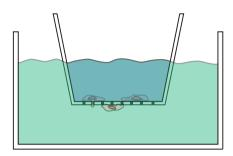
Traditional cell migration analysis methods such as the **Boyden chamber** are end-point methods, and thus have various limitations: The gradients are not well-established or controlled, live cell tracking is not possible and chemotaxis cannot be distinguished from random cell migration.
