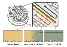
The injected cells adhere and 2D chemotactic cell responses are measured in the gradient region. Non-gradient cell behavior is measured in the control regions.
