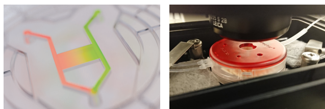
Figure 1. Left panel: A stable small-molecule gradient is formed by diffusion through the polymerised spheroid-matrix mixture inside CellDirector 3D. Right panel: CellDirector 3D set-up in a standard inverted microscope with an incubator stage for temperature and humidity control.
