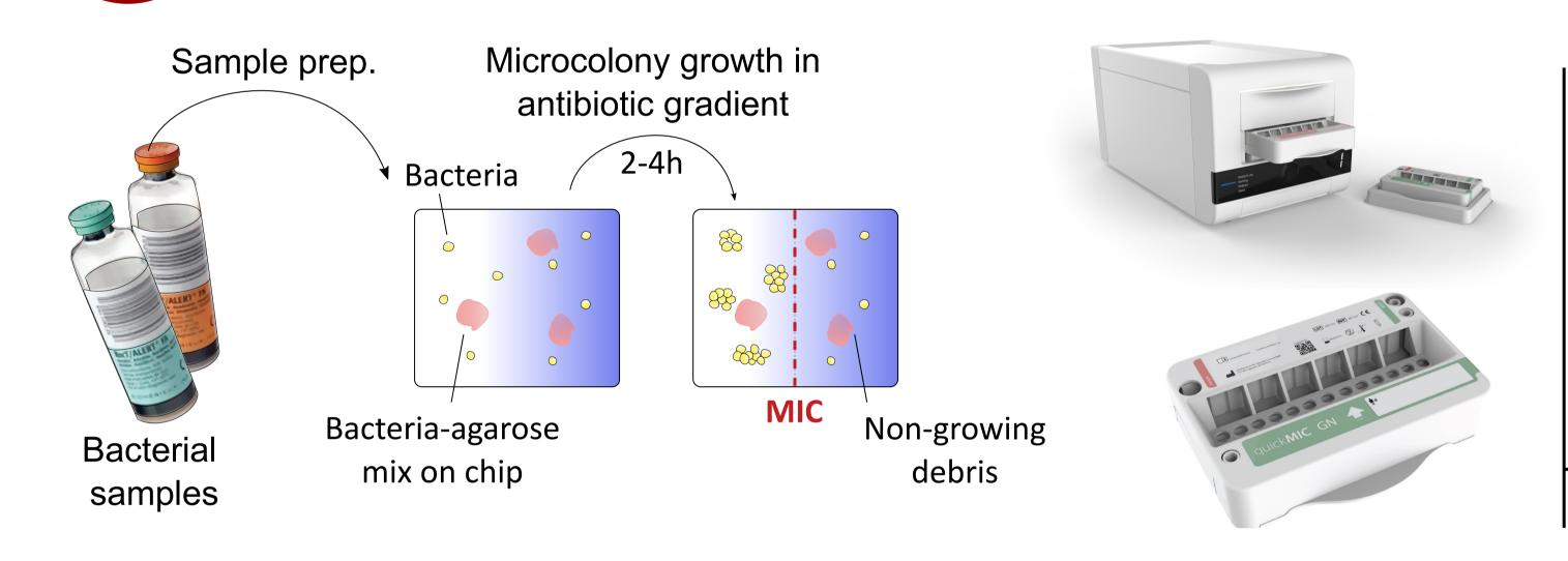
Gradientech AB has developed a new rapid AST system, QuickMIC. The QuickMIC system uses a microfluidic cartridge with 12 different antibiotics, forming gradients through each sample chamber. The QM Analyst read-out software can measure an exact linear MIC within 2-4 hours, directly from blood cultures. This allows rapid categorization of resistance, using EUCAST breakpoints.
